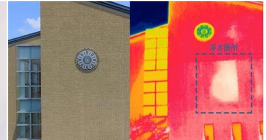
Infrared rays can identify floating tiles
