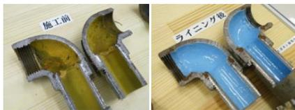
Cleans the inside of the piping and lasts longer due to lining processing
